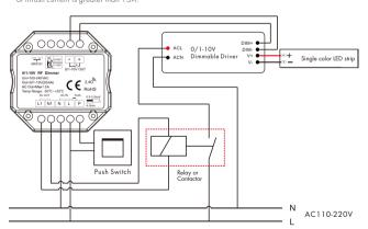
Note: We recommend the number of LED drivers connected to 0/1-10V dimmer does not exceed 20 pieces, The maximum length of the wires from dimmer to LED driver should be no more than 30 meters.
